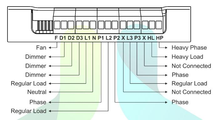
Here Ph indicates Phase (Live wire) input, N indicates Neutral input and HP indicates Heavy Phase input. The loads connected to the different output terminal are described in detail below:
