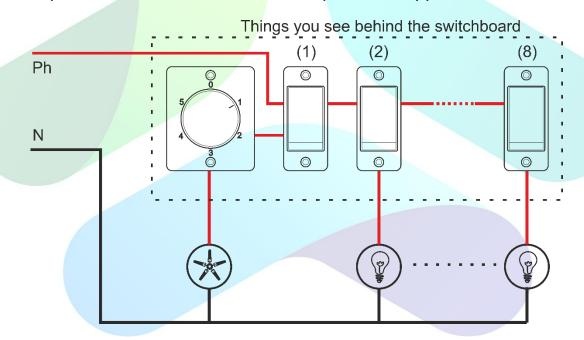
The next wiring diagram gives a basic explanation when a 8.1 device is connected behind a switchboard with 8 switches.
