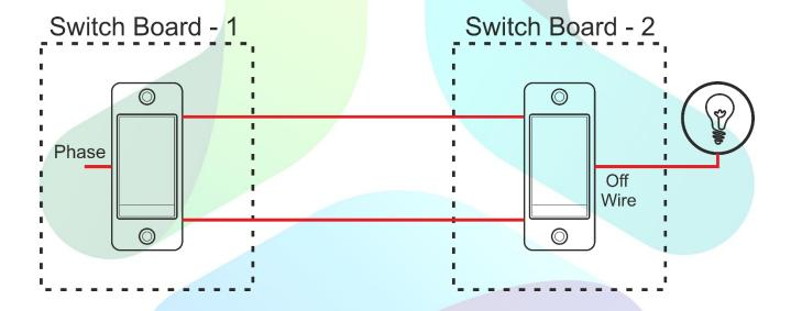
Now, if we install 8.1 with traditional switches and wish to make a two-way connection, then we need to insert an extra wire between the two switchboards. The common black wire from the connector provided should be connected as shown below. If no extra wire exists between the two switch boards, then it is not possible to make a two-way connection.
