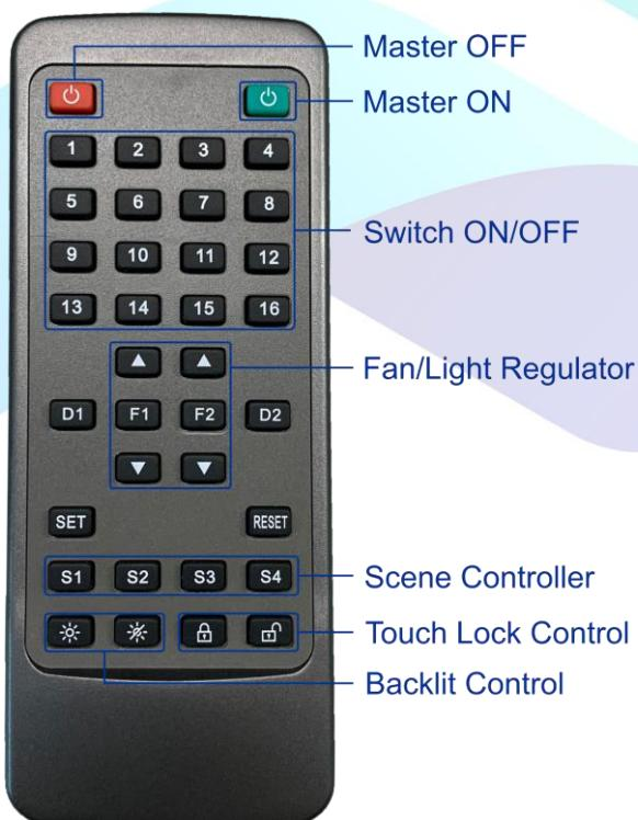
We can turn on/off any load using this remote. We can also set the fan speed or change the brightness of any dimmable light using this remote. Apart from these basic functions, the different types of features which are possible using remote are as follow:
