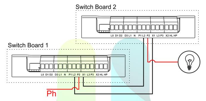
If traditional switches are connected on the other side, then the two-way connection is possible and the wiring diagram will be as follows
