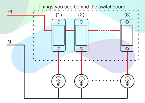
The next wiring diagram gives a basic explanation when a TS.8S is connected with the loads.
