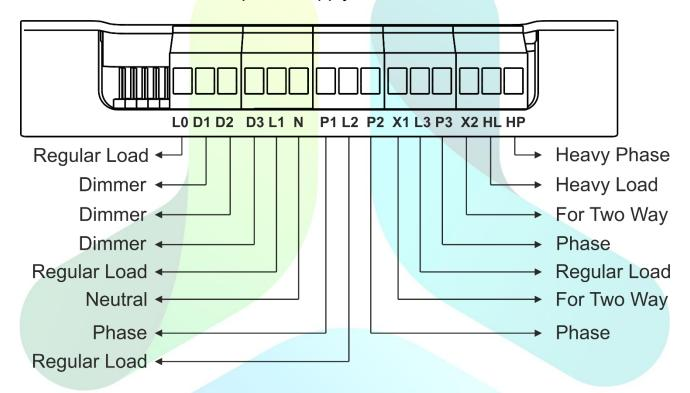
Here Ph indicates Phase (Live wire) input, N indicates Neutral input and HP indicates Heavy Phase input. The loads connected to the different output terminal are described in detail below:
