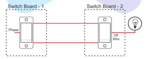
If Smart Node Touch Switches are connected on both sides, then the twoway connection is possible and the wiring diagram will be as follows
